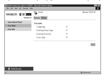
**Config Page** Insert a check mark into the box to print the printer setup page.
