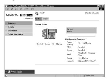
**Device Status** This area uses graphics and text to shows the configuration of options installed on the CF2001P.
